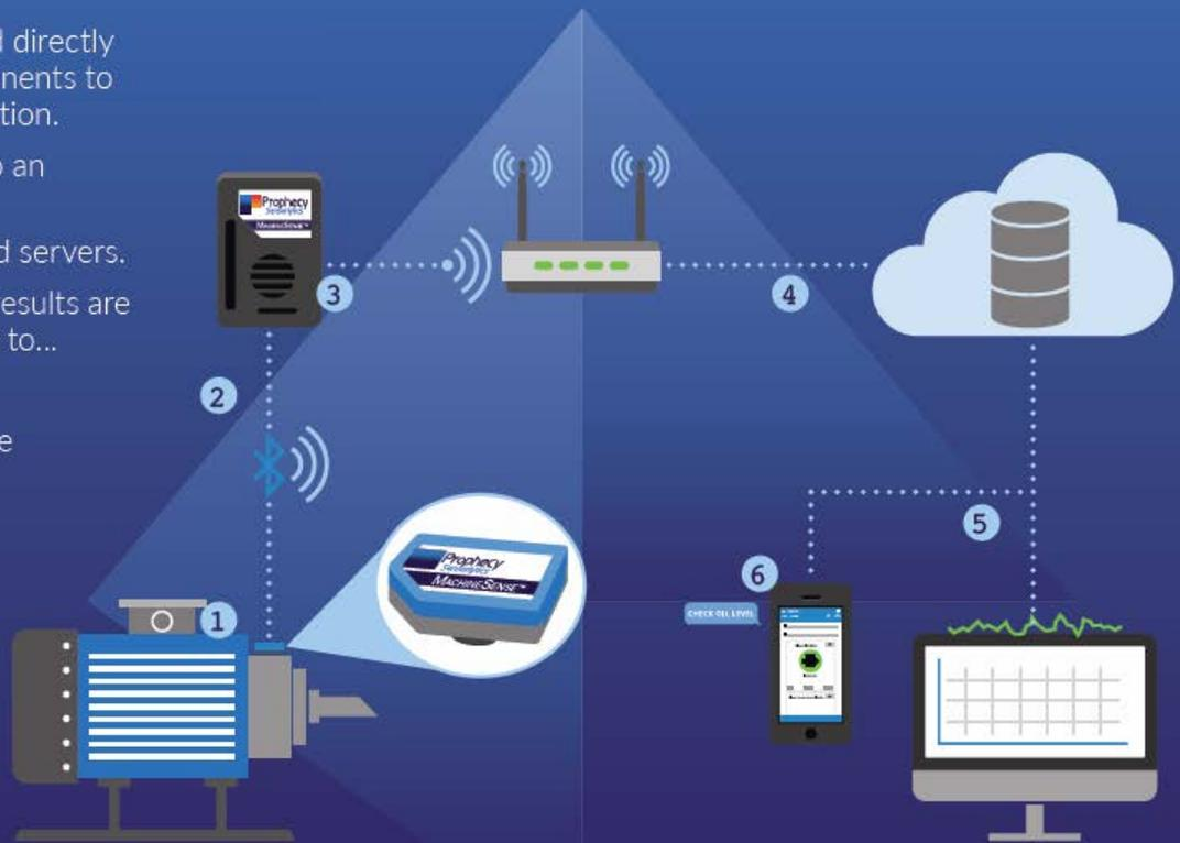
Fig. 2: How MachineSense works in the Prophecy Predictive Maintenance IoT system
